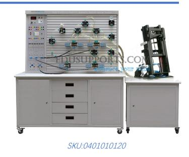
9. **Relay Control Option**: In addition to PLC control, the trainer offers an independent relay control unit. Comparing both methods, students gain deeper insights into the advantages of PLC programmable control and strengthen their understanding of PLC programming.
